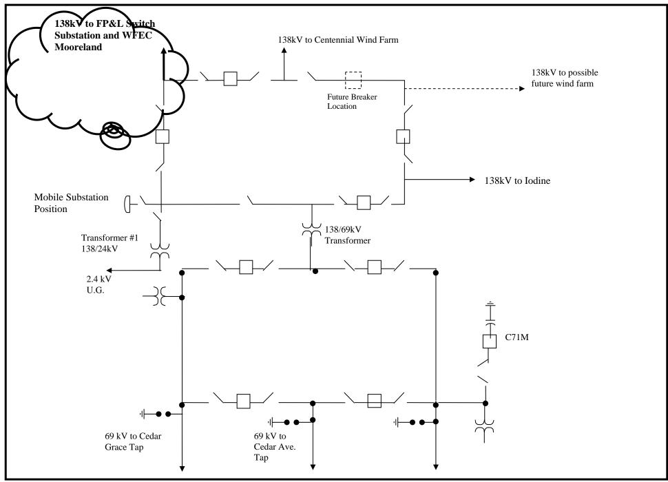
Transmission Line to be Rebuilt From Woodward District Substation to FP&L Switch substation
